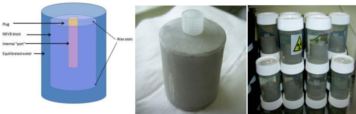
**Figure 1-3: Schematic and photograph of diffusion apparatus**
