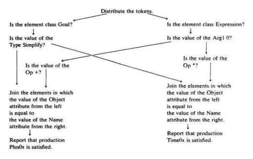
Figure 3.2: Rete Network for Plus0x and Time0x [For82]
