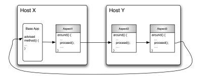
Fig. 6. Around advice chaining in AWED. Advice applicable to the same joinpoint execute in a single advice chain, regardless of execution host.
